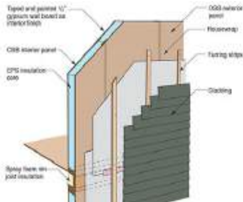
Fig 5 (i) & (ii) Schematic view image of Structural insulated panel technology (Source: buildingscience.com)
